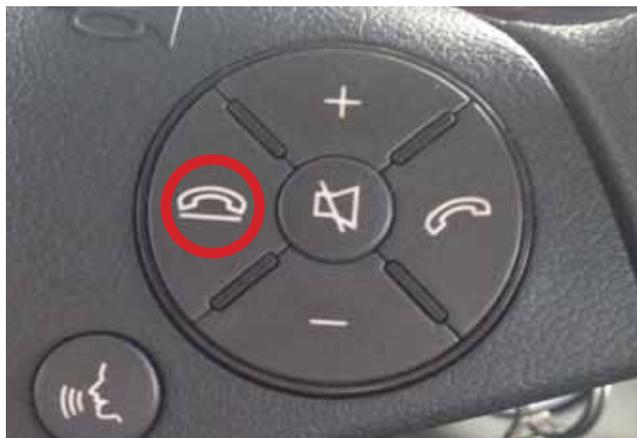
**4** Press the Telephone Hangup button on the steering wheel.
