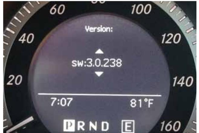
**3** The second Version menu line shows the current software version of the Remote Start Module.
